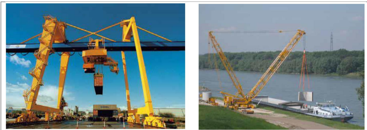
Figure 5: Bridge crane at the port of Krems (source: Mierka Donauhafen Krems)
